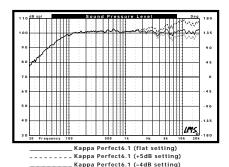
Figure 12. System frequency response
