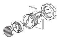
Figure 6. Flush-mounting the tweeter
